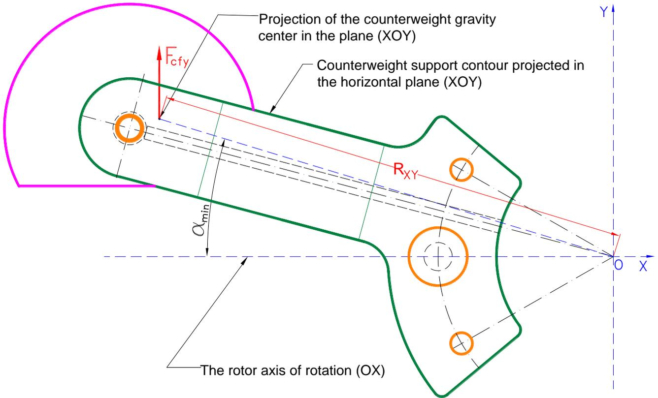
Fig. 3. Projection of counterweight in a plan (XOY)
