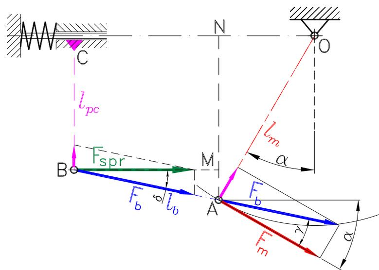
Fig. 5. The decomposition of forces in the slider-crank mechanism
