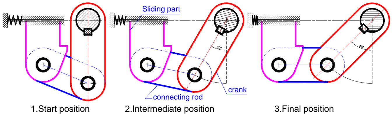
Fig. 4. Three successive positions of the slider-crank mechanism
