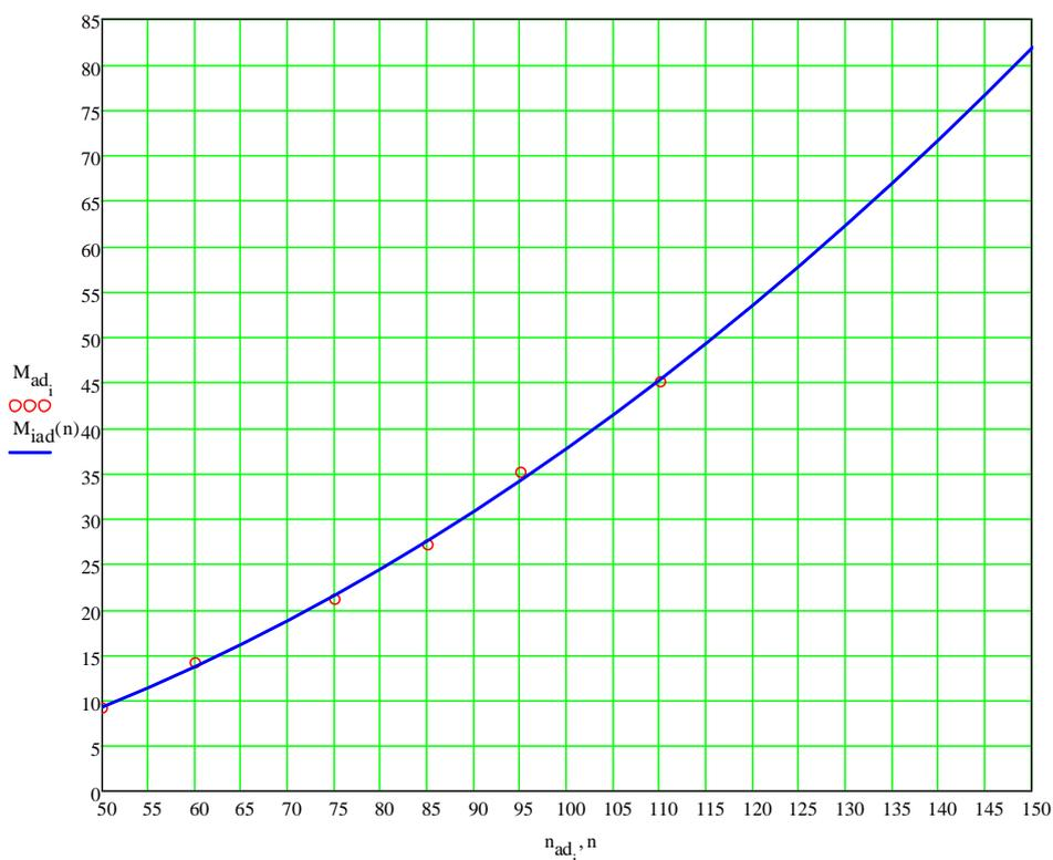
Fig. 6. The aerodynamic torque,  $M_{ad}$ , curve versus rotational speed,  $n$
