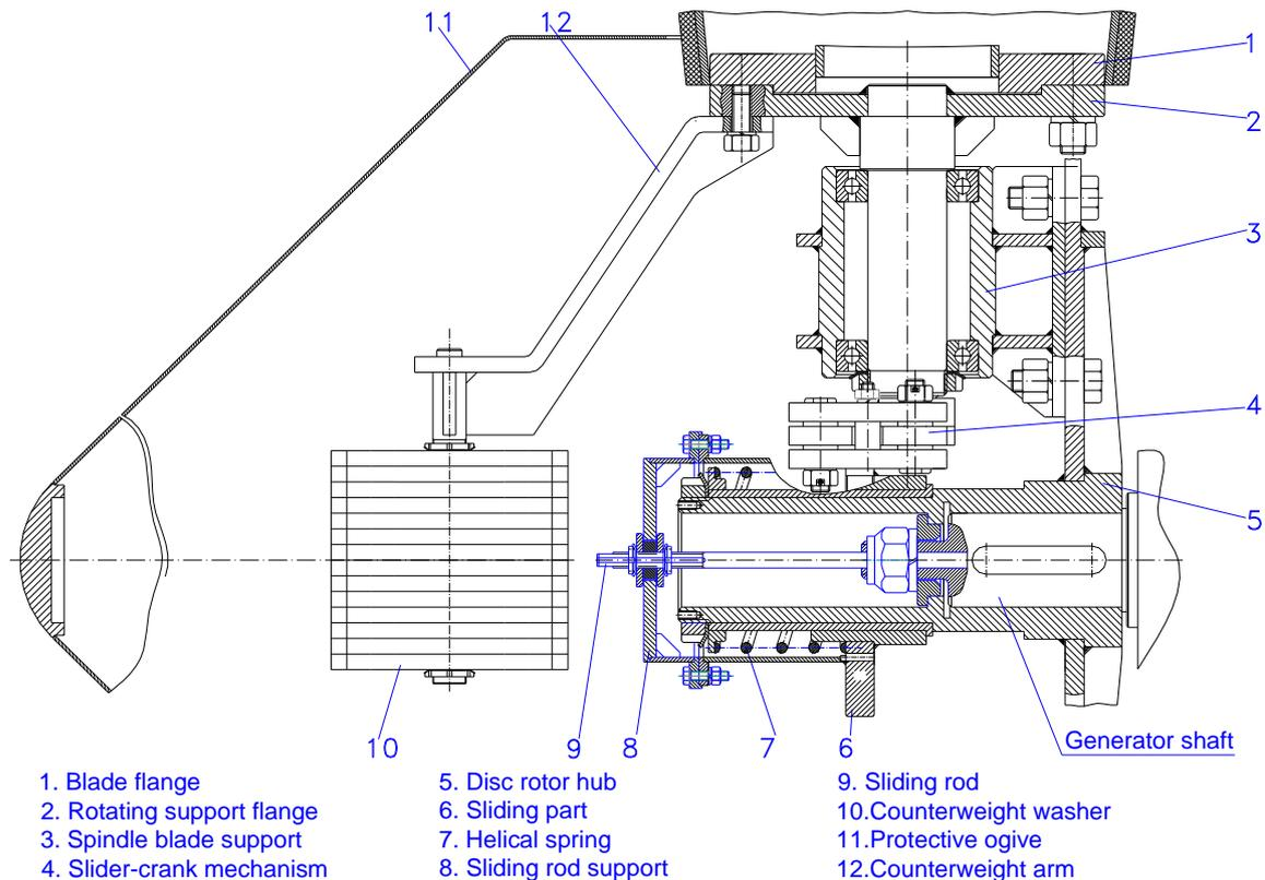
Fig. 1. Centrifugal protection mechanism for over-speed
