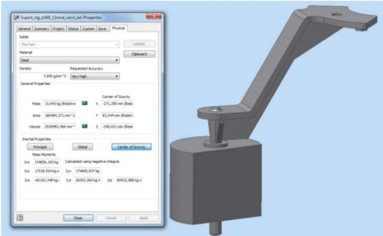
**Fig. 2.** The 3D representation of counterweight and the data plate displayed by the 3D design environment
