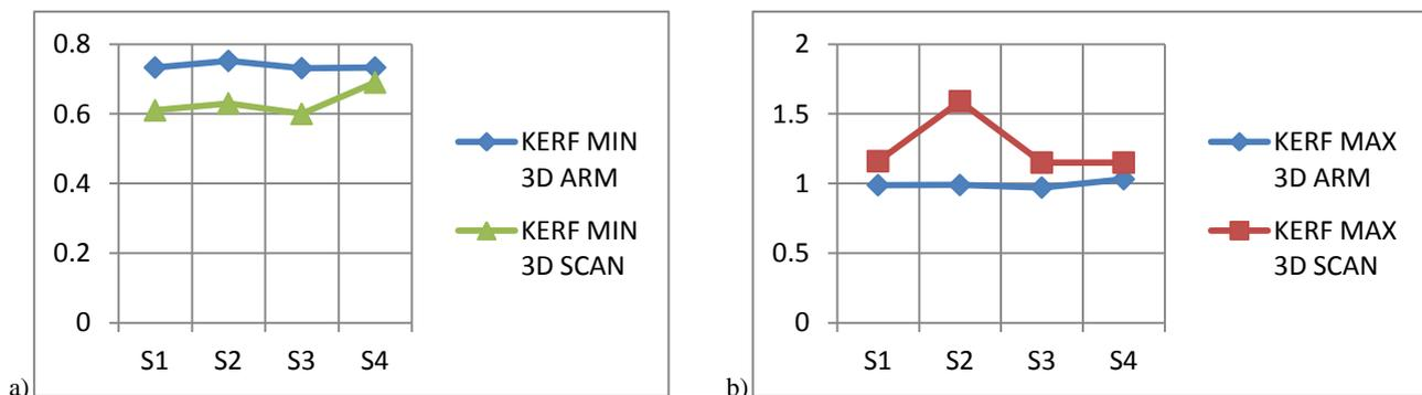
**Fig. 8.** Analysing the kerf width in both of the analysed cases (using the 3D measuring arm and also using the 3D scanner): a) Kerf width minimum values, b) Kerf width maximum values.
