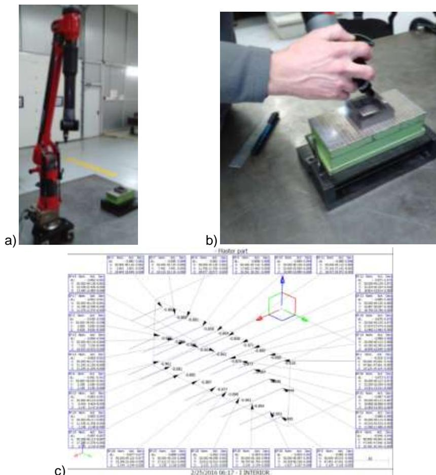
Fig. 5. a) Cimcore Infinite 3D measuring arm, b) Measuring the part, c) The way of measuring the part
