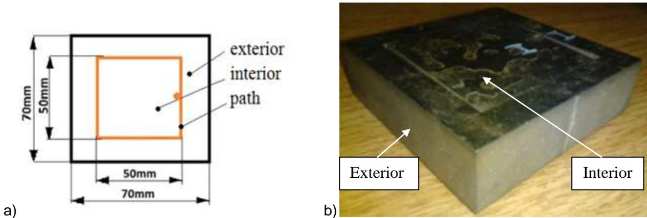
Fig. 2. a) Design for cutting, b)The cutted C45 part
