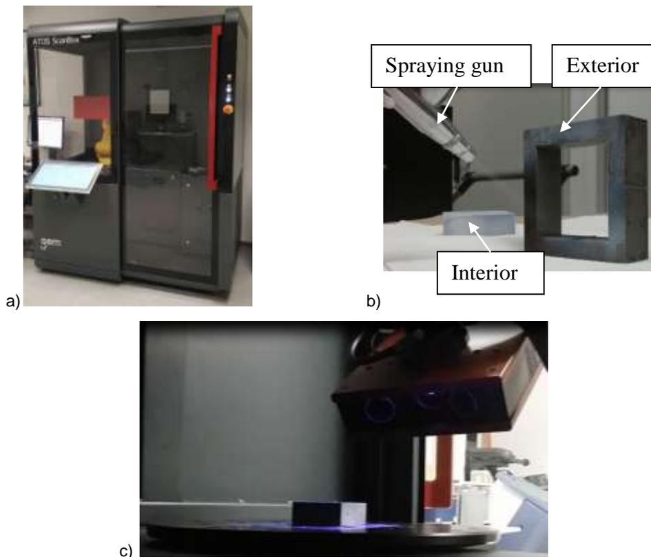
**Fig. 6.** a) GOM ATOS ScanBox 4105, b) Spraying the parts with titanium based spray paint, c) Scanning the parts
