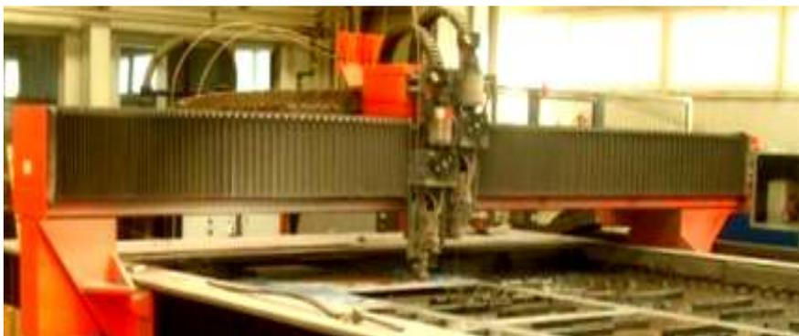
**Fig. 1.** Bystronic ByJet Pro L water jet cutting machine;
