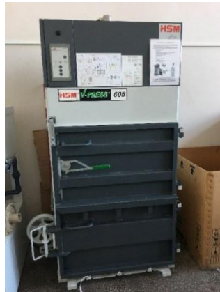
Fig.5. Hydraulic baling press – studied model, available in one laboratory of Faculty of Biotechnical Systems
