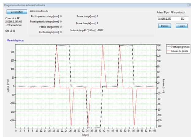
Fig. 10. The operator console – step type input signal
