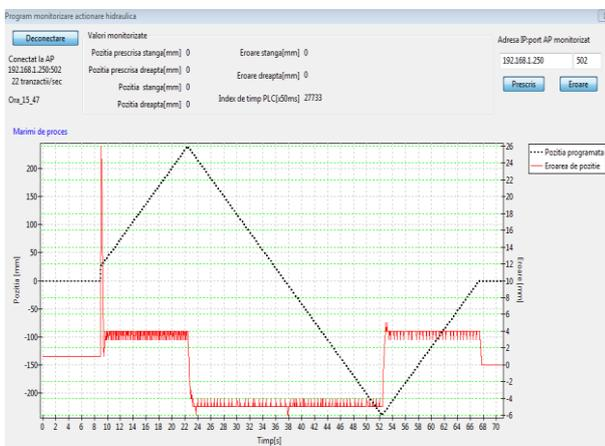
Fig. 9. The operator console – ramp type input signal
