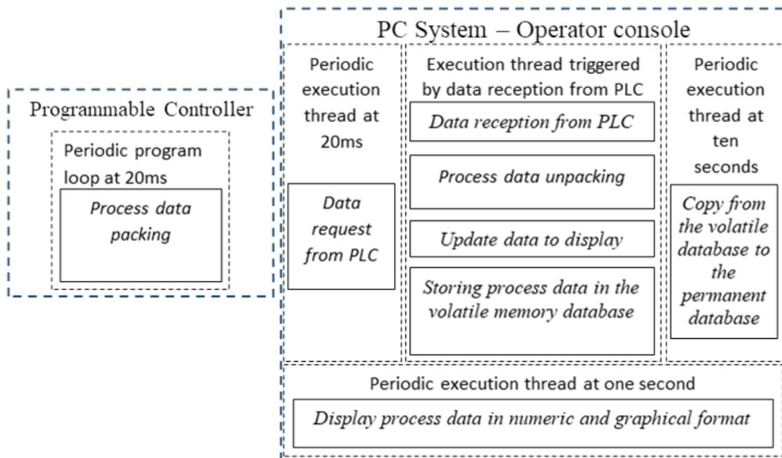
Fig. 2. Software architecture
