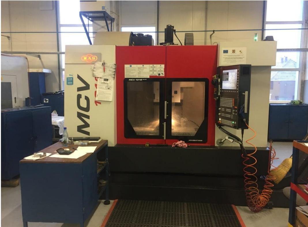
**Fig. 3.** Vertical machining center in 3 axis MCV 1016
