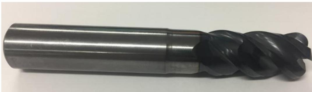
**Fig. 4.** The toroidal milling cutter
