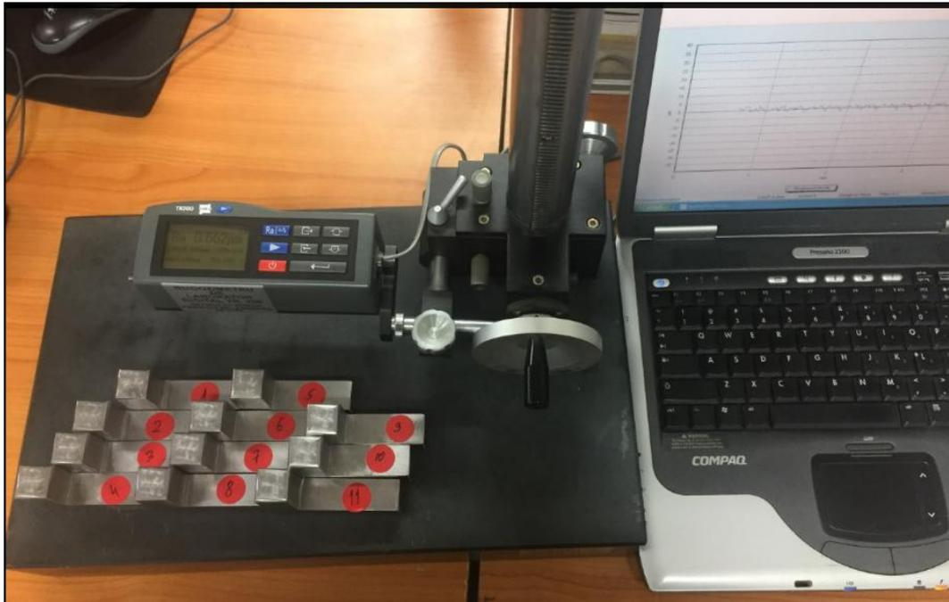
Fig. 7. Roughness measurement with TIM 200 TR
