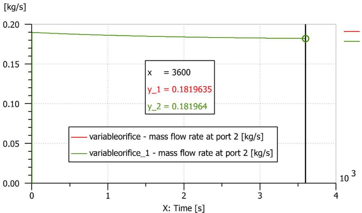
Fig. 10. Mass flow through the hydraulic orifices (throttle)
