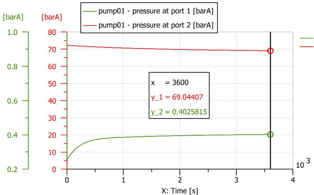
Fig. 8. The pressure developed at the inlet and discharge of the hydraulic pump
