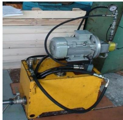
Fig. 2. Experimental bench for hydrostatic pump testing [2]
