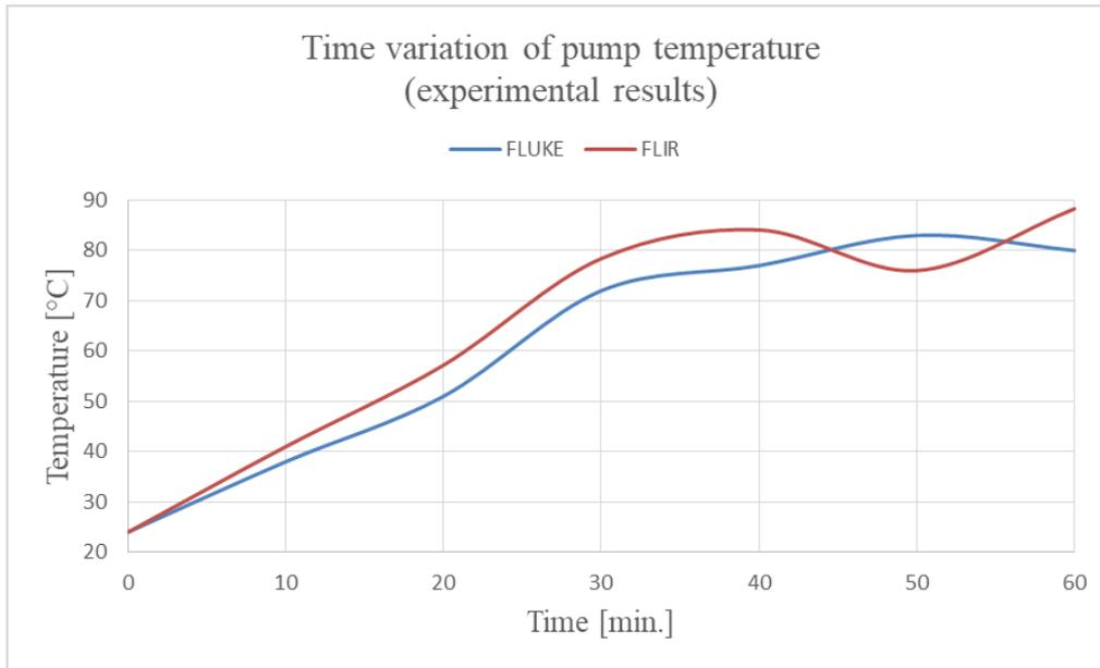
**Fig. 6.** Trend graph of measured temperatures with Fluke IT and FLIR IC
