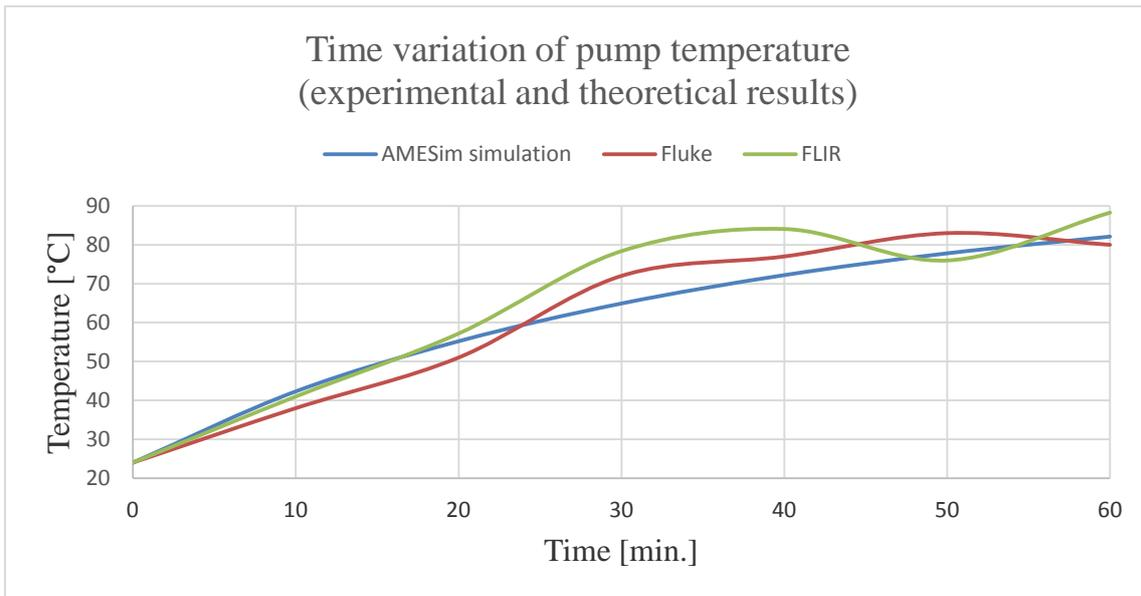
Fig. 14. Hydrostatic pump temperature
