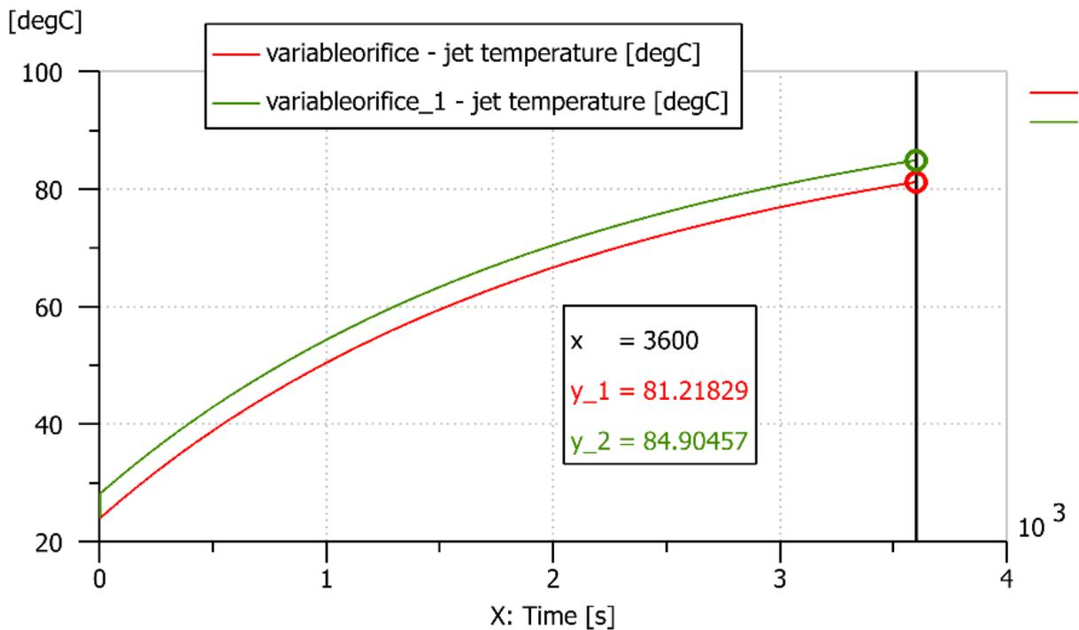
Fig. 12. Liquid stream temperature through the hydraulic orifices (throttle ST and RT)
