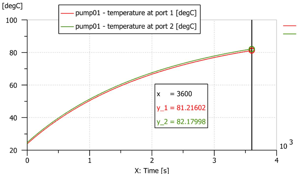
Fig. 13. Fluid temperature in pump inlet and discharge
