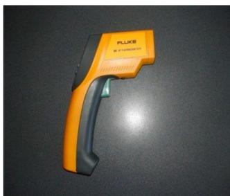
Fig. 3. Fluke infrared thermometer
