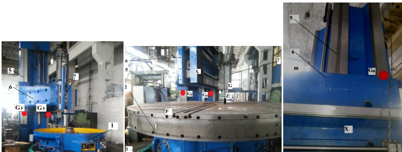
Fig. 10. Front guideways ( G_F ) and back guideways ( G_B ) of the cross-rail on the column that are adjusted by means of the closing gibs
