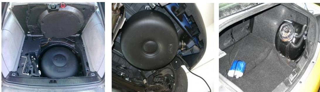
Fig. 1. Different locations of the pressurized toroidal LPG fuel tanks
