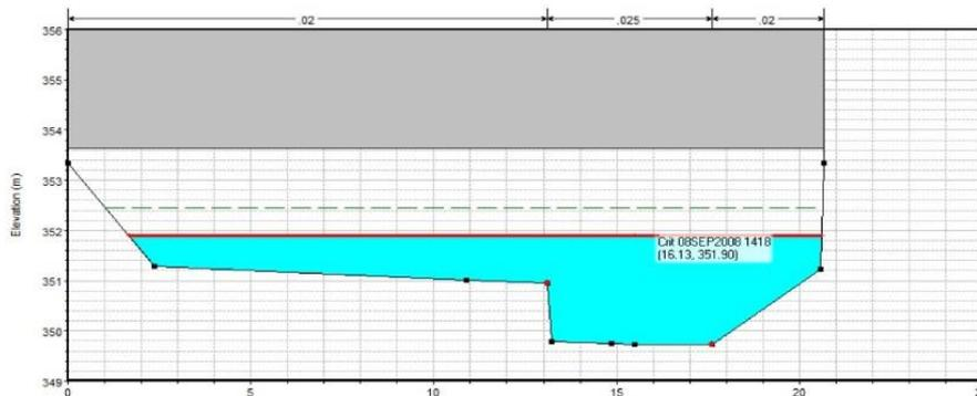
Fig. 8. Upstream Rusor River cross section at railway bridge, natural river flow regime scenario
