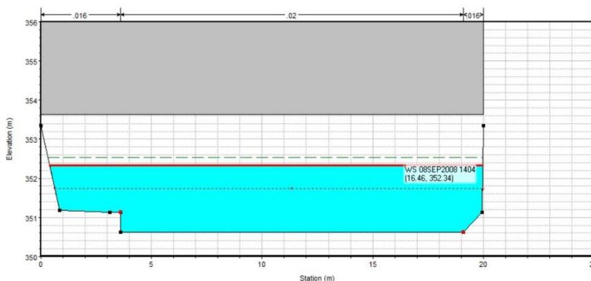
Fig. 11. Upstream Rusor River cross section at railway bridge, regularised river flow regime scenario
