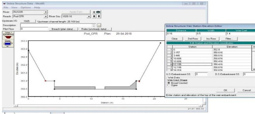
Fig. 5. River cross section at bottom weir, Rusor River
