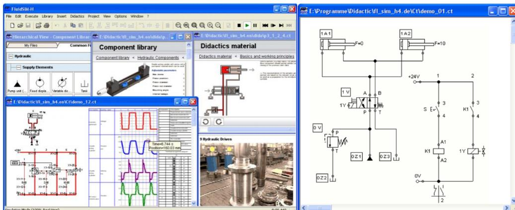
Fig. 3. FluidSIM Hydraulics modeling and simulation environment [7]
