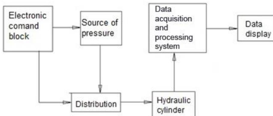
**Fig. 3.** Block diagram of the pellet stand
