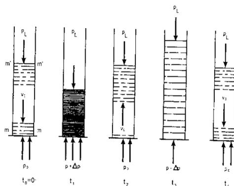
Fig. 3. Pressure oscillations [1]
