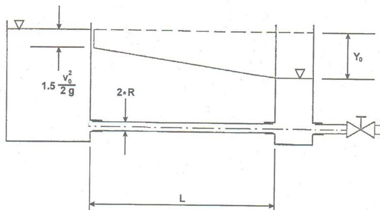
Fig. 1. Scheme of tank and the piezometric tube
