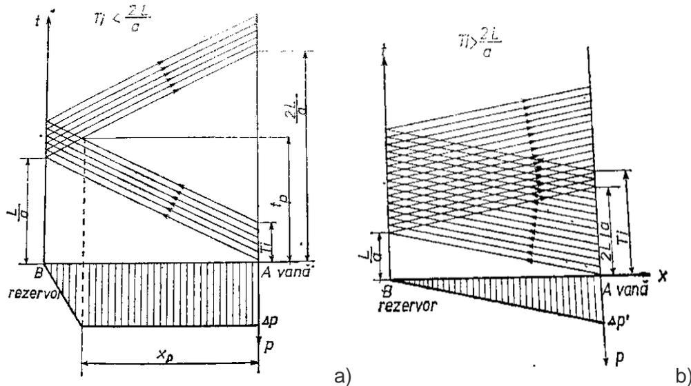
Fig. 4. The phenomenon of the water hammer at the sudden and slow closure of the valve,  $L$ -closure time, a water velocity [1]
