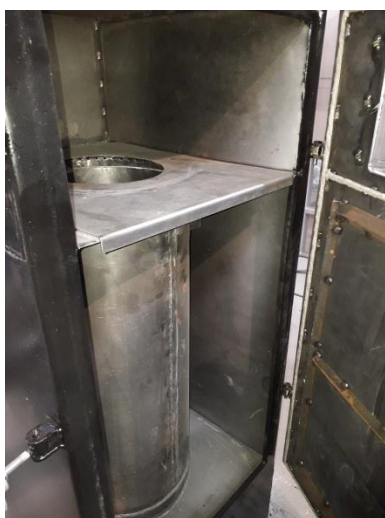
Fig. 10. The TLUD heat generator reactor
