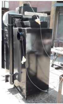
Fig. 5. TLUD thermal generator prototype equipped with heat-resistant for temperature monitoring at points of interest
