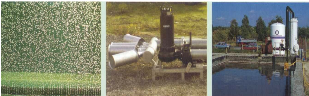
Fig. 4. The charging procedure developed by Messer for pure oxygen: gas hose (left), injectors (center), oxidizer (right) [7]
