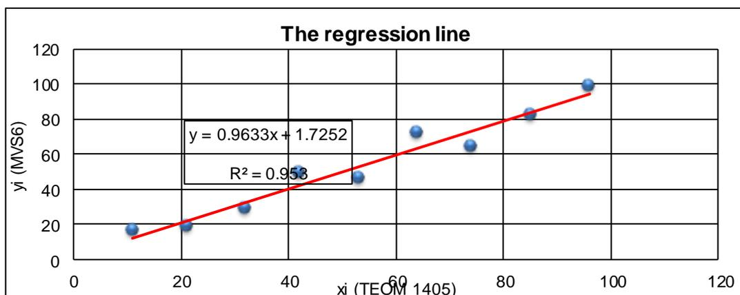
**Fig. 6.** Correlation between TEOM 1405 and MVS6 sampling devices.
