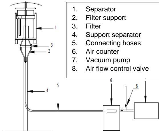
**Fig. 4.** Overview of the MSV6 sampler [12]
