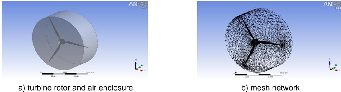
Fig. 3. Analysis main domains and mesh network
