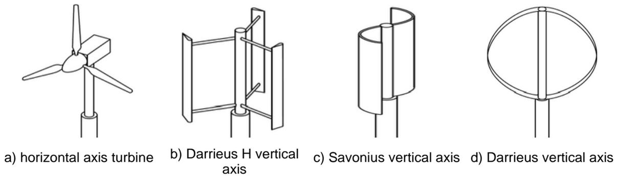
Fig. 1. Principal wind turbine constructive types [8]
