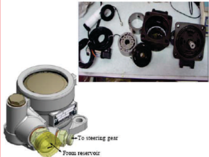
Fig.1. Vane pump with double effect
