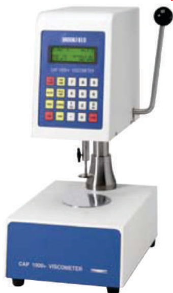
Figure 1: Brookfield cone and plate viscometer, [5]
