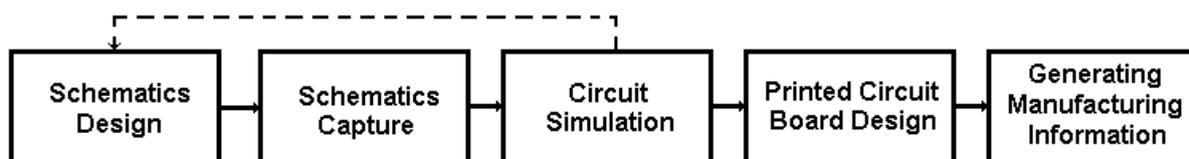
Fig.1 Typical hardware development tool chain
