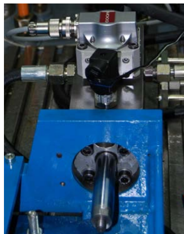
Figure 4 – Example of a servovalve mounted on the computerized stand
