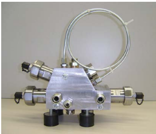
Figure 5: HBC prototype and its steady state efficiency results; (system data: inductance pipe: length: 1.2 m, diameter 3 mm, oil: Shell Tellus 15 cSt @ 40°C; switching valves: LCM FSVi (QN=10 l/in @ 5 bar); switching frequency: 100 Hz; accumulators: piston accumulators, developed by the authors; find all data in [22] and [24]).
