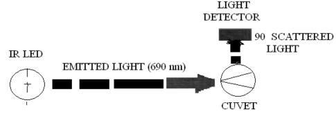
Figure 1 Switching the light beam through the cuvette [1]
