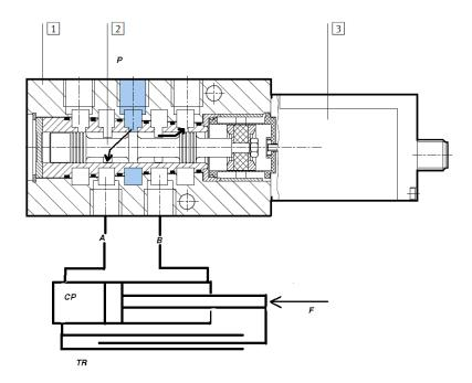
Fig. 1 Directional control valve by FESTO. 1- aluminum body, 2 – aluminum slide valve, 3- electromagnet actuated at amperage 4-20 mA or voltage 0-10 V DC
