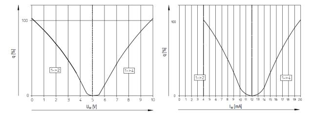
Fig. 3 Flow rate of proportional directional control valve q (%) depending on the control voltage (left) and amperage (right)
