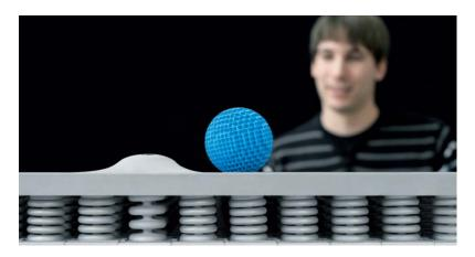
Fig. 5 The way the pneumatic cylinder operates on the conveyor membrane
