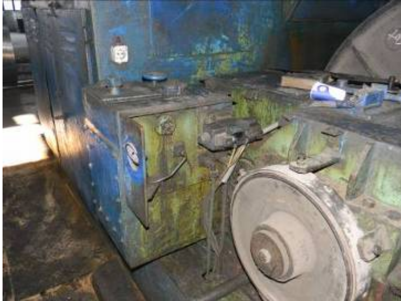
Fig.5. The existing pumping unit and the shoe and drum brake of the reducer: there have been blocked the pipes by which this group supplies the hydraulic cylinder of the reel; a speed transducer was mounted on the drum shaft of the reducer.
