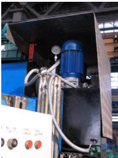
Fig.6. The modular pumping unit fitted with proportional directional control valve (IHP).
