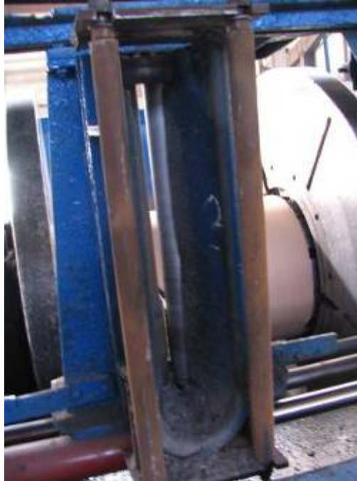
Fig.3. Reeling head, driven by a hydraulic cylinder with fixed bilateral rod and mobile liner.
