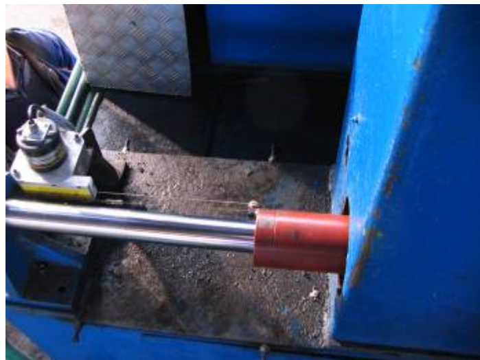
Fig.7. Drive cylinder of the reel: position and speed cable transducer (IHP).
