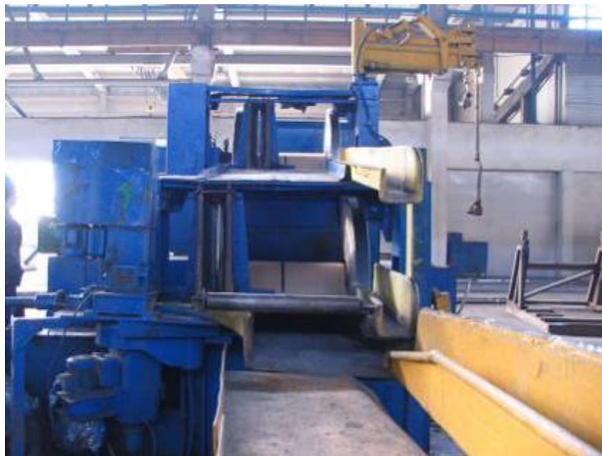
Fig.2. Two drum coil winding machine idle: both reels stationed at the flange on the left of drums; right, foreground –gutter through which the wire comes from the rolling mill; right, background - gutters through which the wire is directed to the drums, where it is taken up by the reel.
