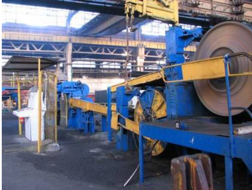
Fig.1. Wire production flow (back to front): furnace, rolling mill, gutter, winding machine with two drums and two reels.
