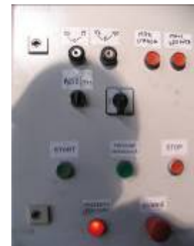
Fig.10. The outside of the board case (IHP): wire diameter selection keys; reel manual displacement control; operating mode switching control; start; stop; signaling lamps.
