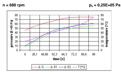
Fig. 3 Diagram of pressures and temperature variation with time in static pressure of 0,25E+05 Pa
