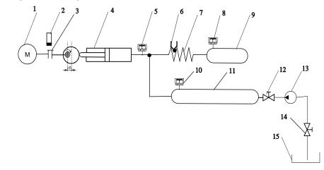
Fig.1 Block diagram of unconventional installation
