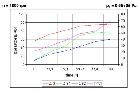
Fig.5 Diagram of pressures and temperature variation with time in static pressure of 0,5E+05 Pa
