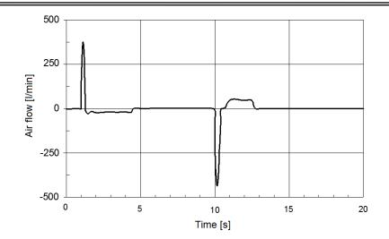
Figure 5 – Air flow variation diagram in the pneumatic actuator (9).
