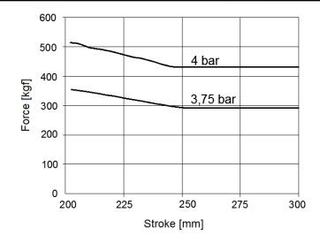
Figure 1 - Characteristic diagram of the pneumatic spring.
