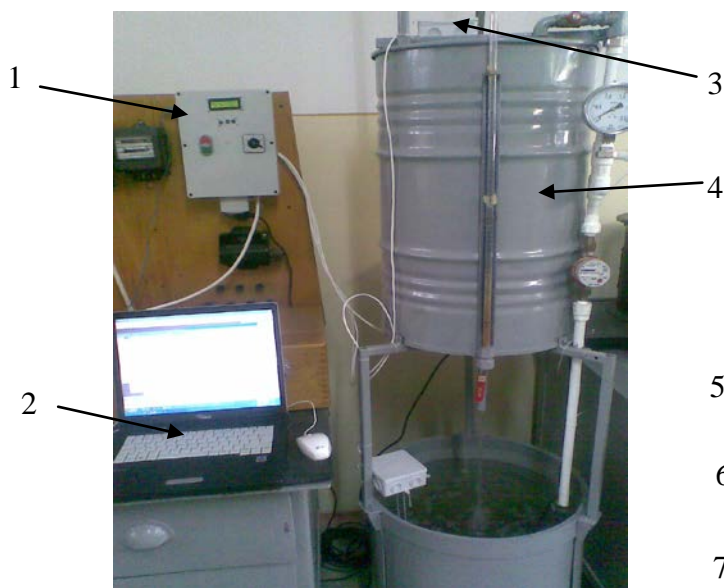
Fig. 8. Automated pumping system: 1- automation box; 2- laptop (PC); 3- sensors box of storage tank; 4- storage tank; 5- sensors box of supply tank 6- submersible pump; 7- supply tank.
