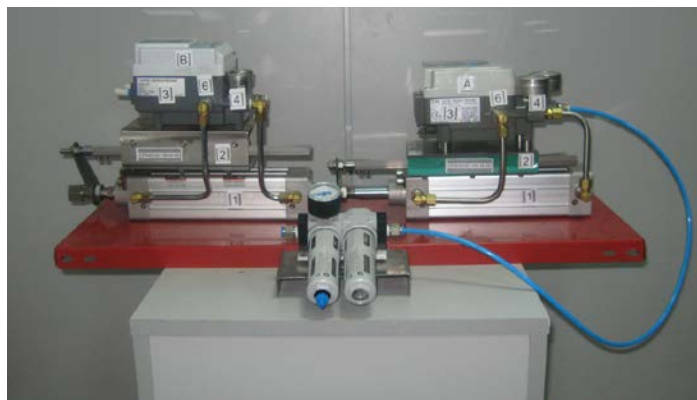
HYDRAULIC DIAGRAM Test stand for a high pressure pneumatic actuator 4.0 MPa
