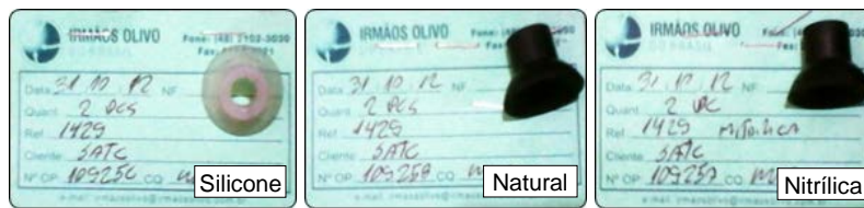
Fig.3. Model and types of suction cups used
