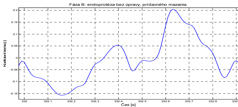
Fig.9 Phase B, Coefficient of friction, endoprosthesis with dry friction
