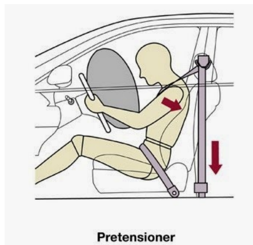
Fig.1. Pretensioning role during a car crash [3]
