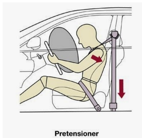
Fig.1. Pretensioning role during a car crash [3]
