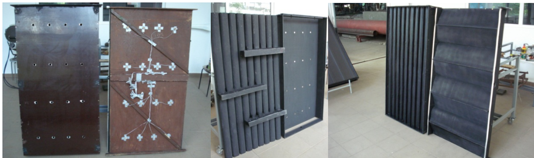
Fig.2 The thermal transducers for both solar thermal air collectors
