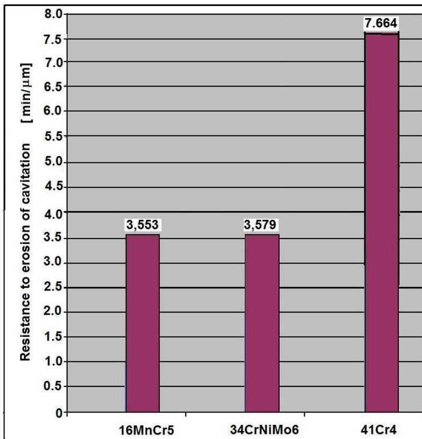
Fig. 6. Comparison of the resistance to erosion of cavitation
