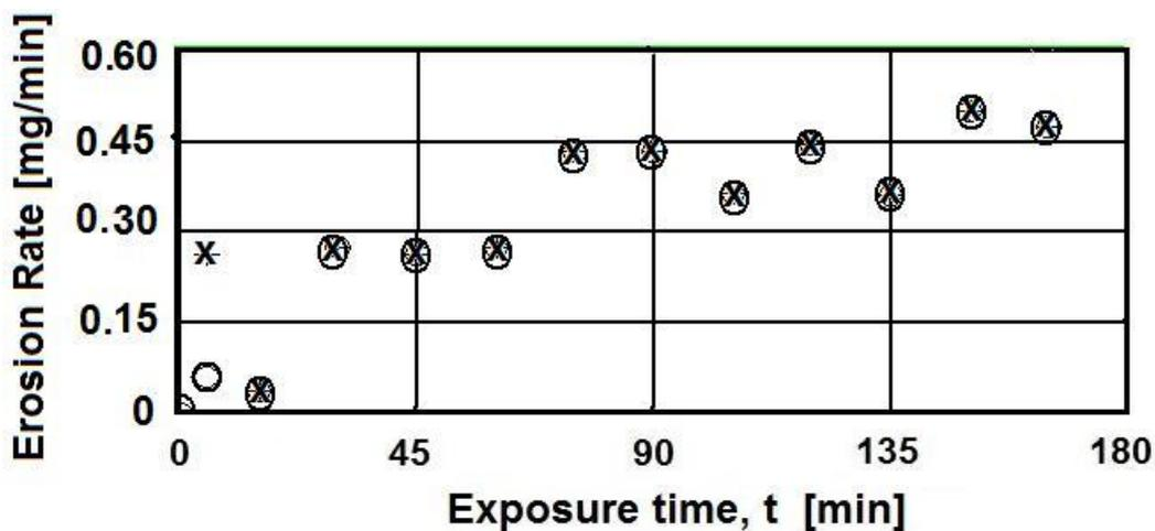
Fig. 2. Dispersion of the erosion rates during the periods of cavitation attack
