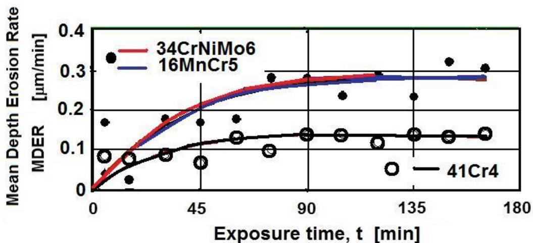
Fig. 4. Mean depth erosion rate with the duration of cavitation attack
