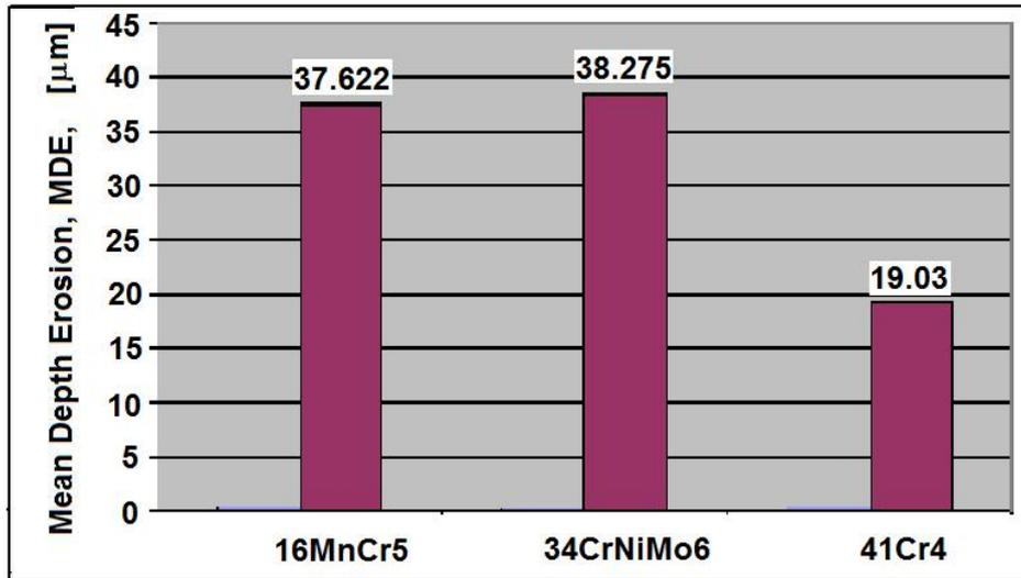
Fig. 5. Comparison of the mean depth of erosion recorded at the end of the test
