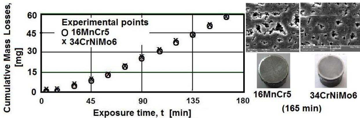
Fig. 1. Evolution of the weigh loss (cumulative) with the duration of the cavitation attack
