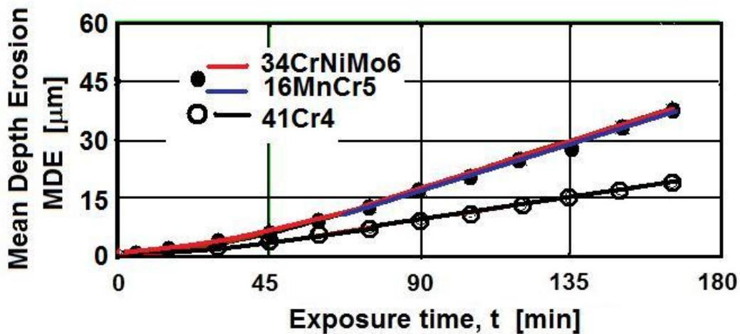
Fig. 3. Mean depth erosion with the duration of cavitation attack
