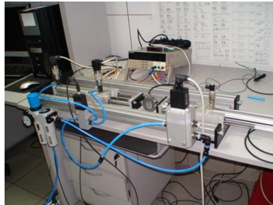
Fig. 3. Pneumatic drive system with medium and high pressure actuators, with pneumatic spring type load
