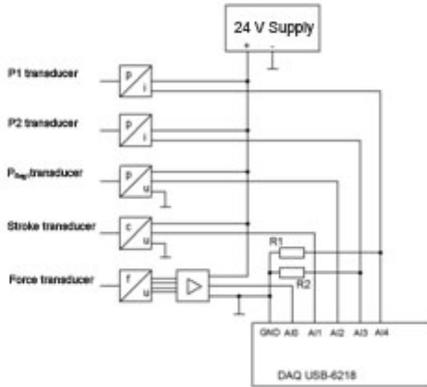
**Fig. 4** Layout of the system for data acquisition from transducers
