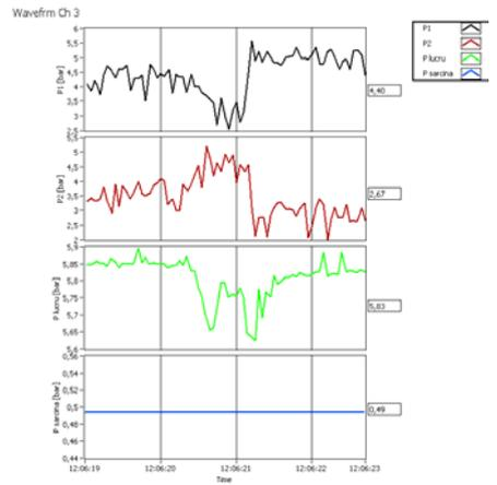
Window displaying the pneumatic parameters of the drive actuator: pressure in piston chamber  $p_1$  [bar], pressure in rod chamber  $p_2$  [bar], working pressure  $p_l$  [bar], load generating pressure  $p_s$  [bar]
