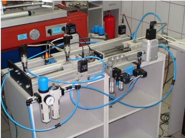
**Fig. 2** Pneumatic system with medium pressure actuators, with load controlled by proportional pressure regulator valve
