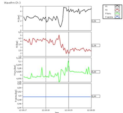
Window displaying the pneumatic parameters of the drive actuator: pressure in piston chamber  $p_1$  [bar], pressure in rod chamber  $p_2$  [bar], working pressure  $p_1$  [bar], load generating pressure  $p_s$  [bar]
