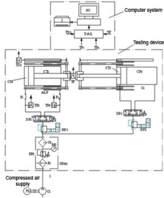
**Fig. 3** Pneumatic diagram of the drive system
