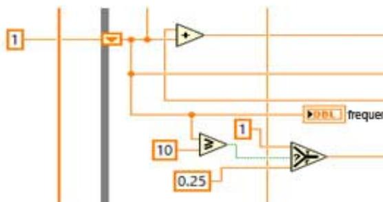
Fig. 7a Generating of frequency pitches (increments) for testing
