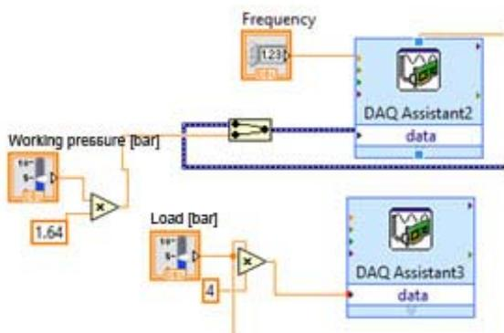
Fig. 6a Control block for proportional pressure regulators
