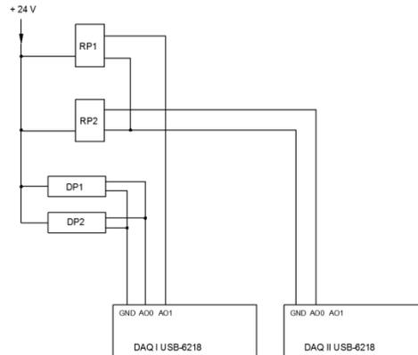
**Fig.5** Control diagram of proportional directional control valves and pressure regulators
