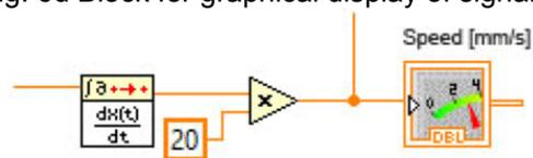
Fig. 6f Speed calculation block
