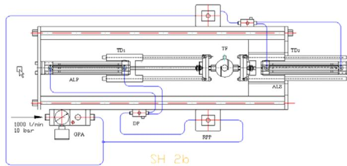
Fig. 1 Drive system with medium pressure pneumatic actuators
