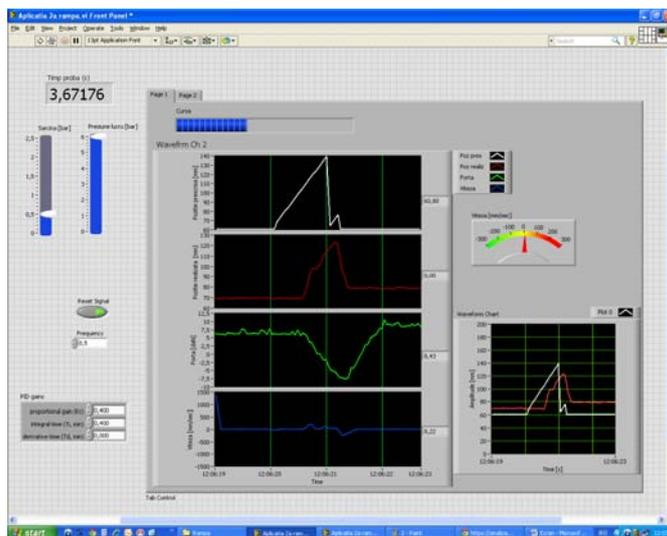
Screen capture highlighting the ramp signal parameters: prescribed position [mm], achieved position [mm], amplitude [mm], pneumatic parameters of the drive actuator: working pressure  $p_l$  [bar], load generating pressure  $p_s$  [bar], parameters of the PID automatic controller:  $k_c$ ,  $T_i$ ,  $T_d$
