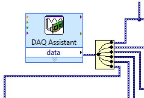
Fig. 6b Block for reading signals from the transducers connected to the inputs AI0...AI4
