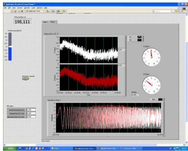
**Fig. 11.** Window 2 of the application - DNCKE-100-200-PPV-A medium pressure pneumatic actuator
