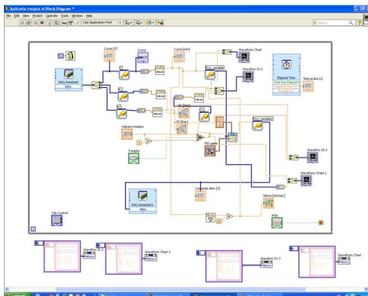
Fig. 5. Software diagram for determining response to step signal, developed in LabVIEW
