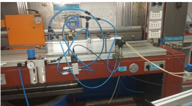
**Fig. 1.** Bench for testing the DNCKE-100-200-PPV-A medium pressure actuator
