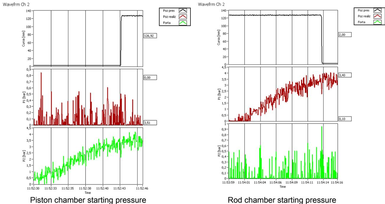
**Fig. 15.** Graphs of starting pressure for the DNCKE-40-130-PPV-A actuator
