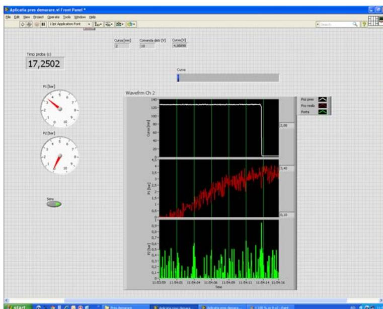
Fig. 14. Window of the application for determining the starting pressure - DNCKE-40-130-PPV-A actuator
