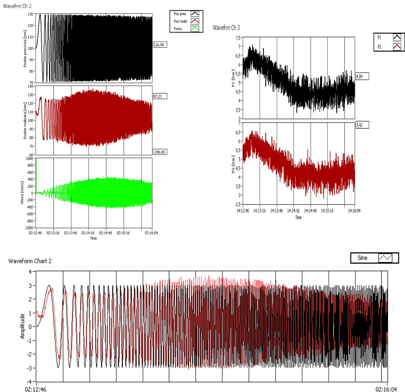
**Fig. 12.** The shape of graphs obtained during tests concerning the response of the DNCKE-100-200-PPV-A medium pressure pneumatic actuator to sine wave signal
