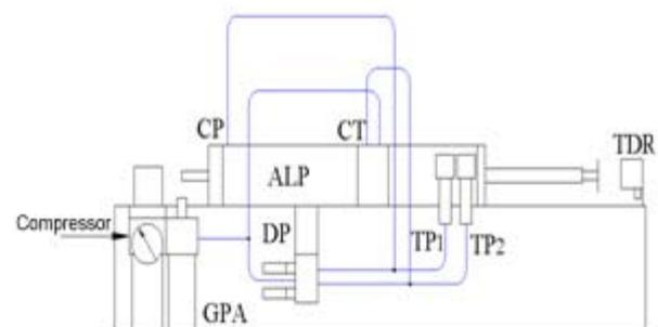
**Fig. 2.** Pneumatic circuit diagram of the test bench in dynamic regime
