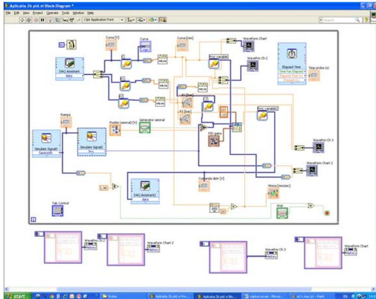
**Fig. 9.** Software diagram for determining the response to sine wave signal, developed in LabVIEW
