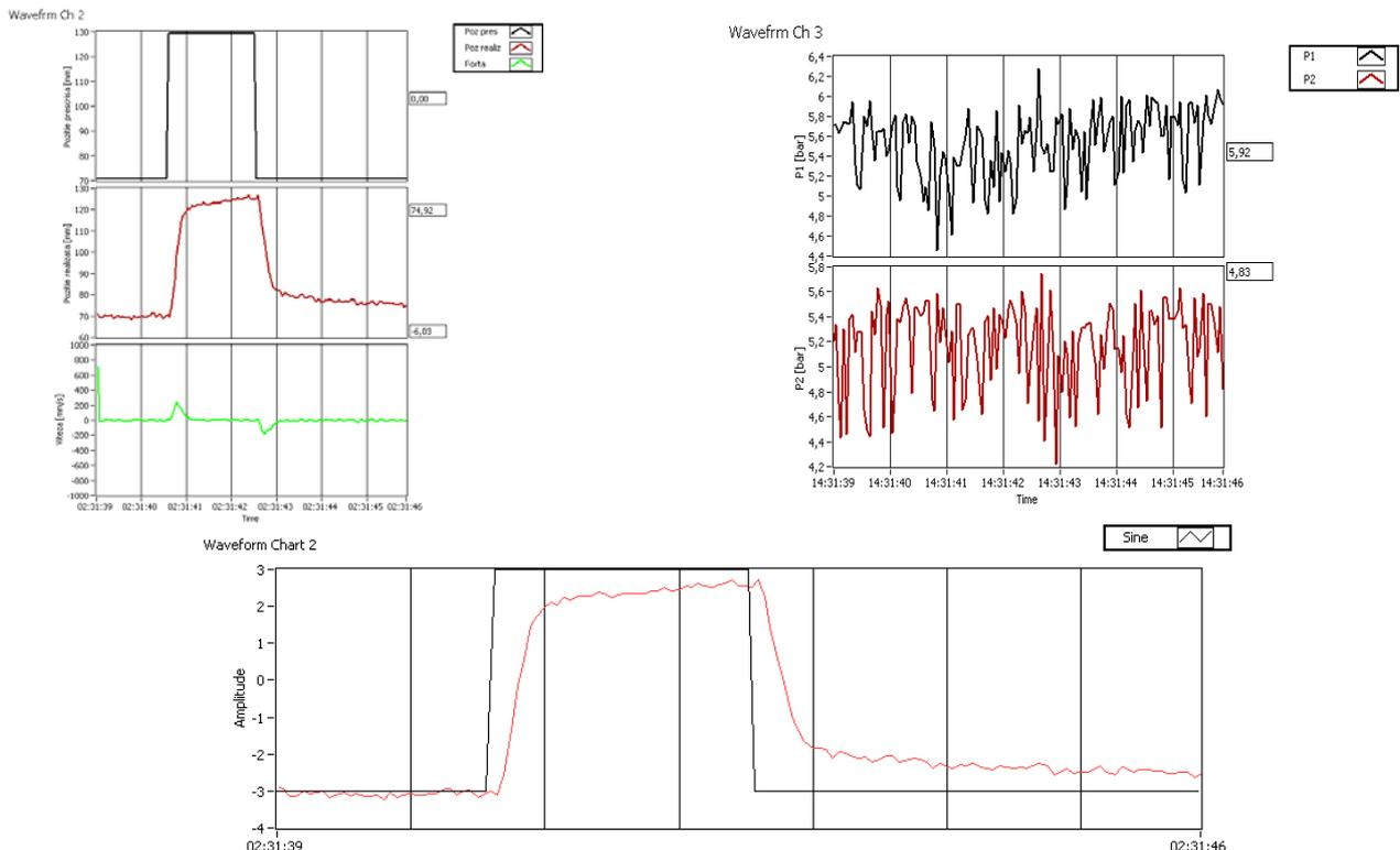
Fig. 8. The shape of graphs obtained during tests concerning the response of the DNCKE-100-200-PPV-A medium pressure pneumatic actuator to step signal
