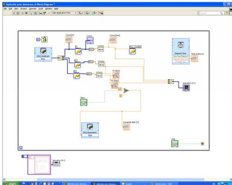
Fig. 13. Software diagram (graphics) for determining the starting pressure
