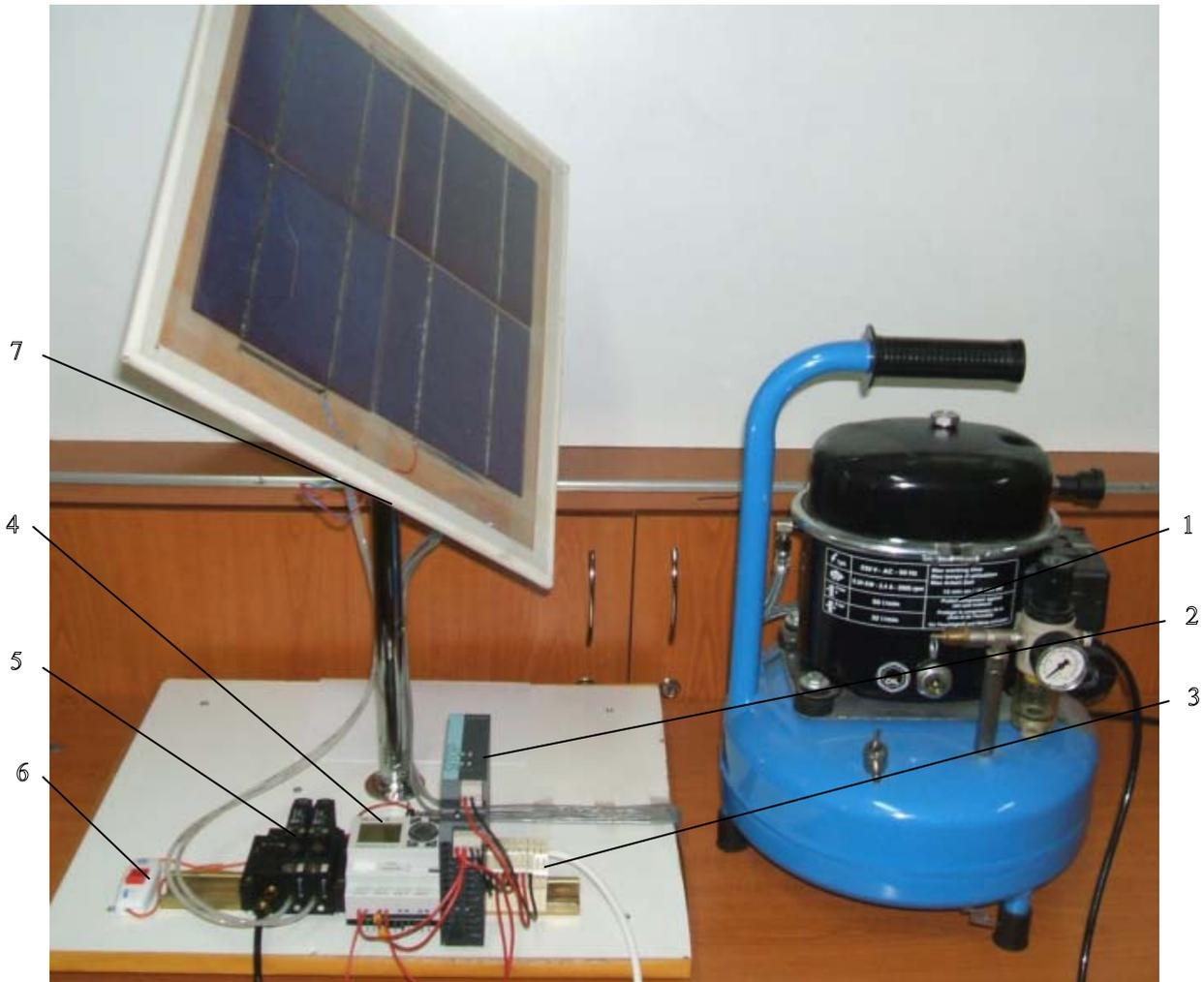
**Fig. 3.** Experimental model of tracking system – electrical part:
