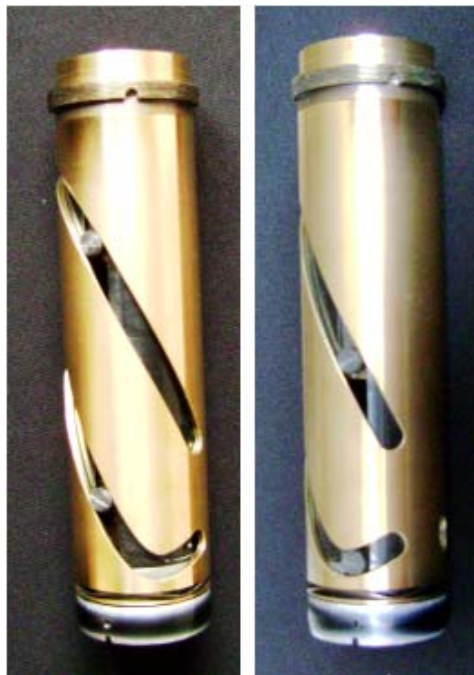
Fig. 3. Zoom system sub-assembly: cam barrel
