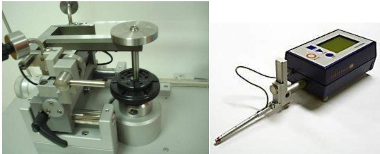
Fig. 6. Tribometer mechanism (left) and profilometer (right)
