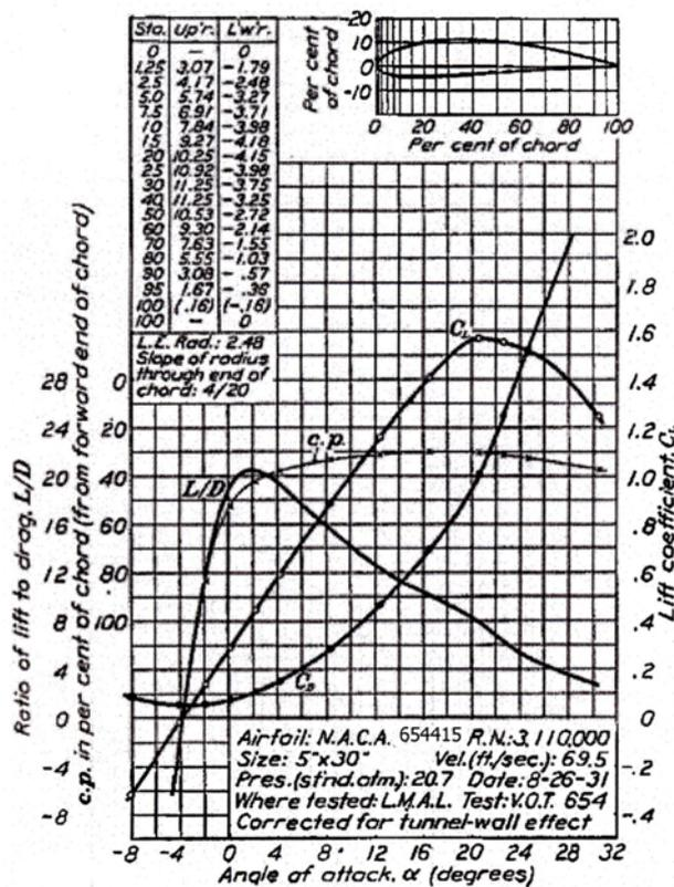
Fig. 9. Characteristic curves of the NACA 654415 profile
