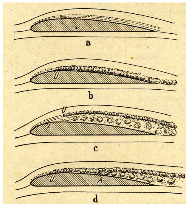
**Fig. 4.** Development of the boundary layer and the flow separation from a blade:
