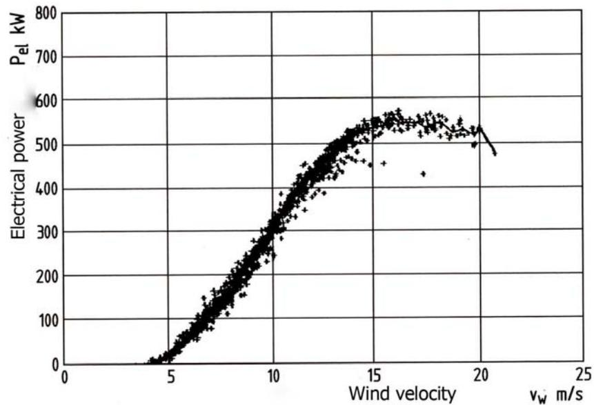
**Fig. 5.** Mean measurements, with 10 minutes rate, power in function of wind velocity at a wind turbine with fixed blades and with the limiting power through flow separation of the flow from the blade (stall).
