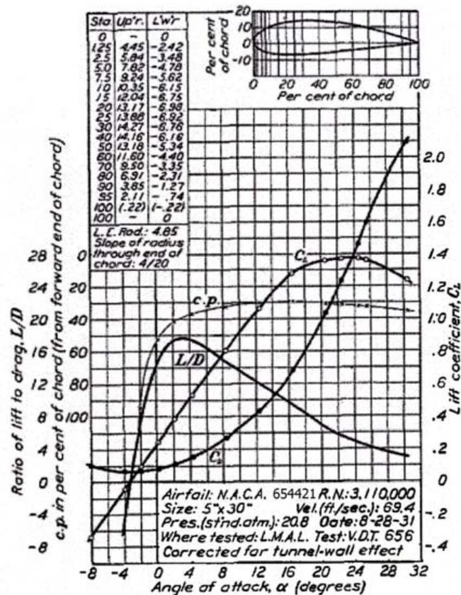
Fig. 11. Characteristic curves of the NACA 654421 profile
