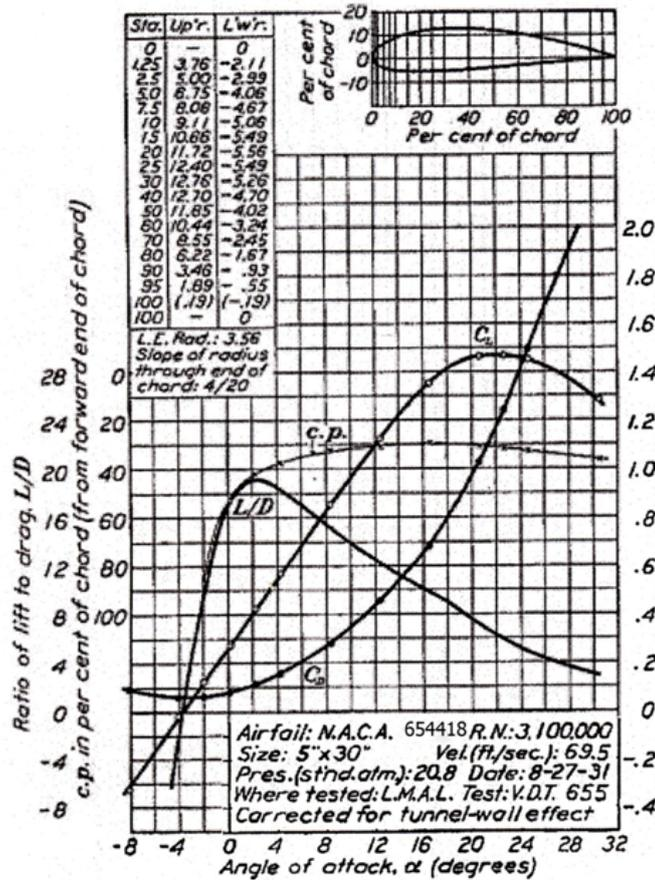
Fig. 10. Characteristic curves of the NACA 654418 profile
