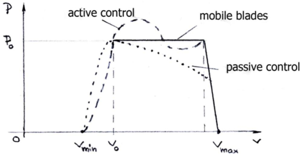
Fig. 1. Passive and active control of separation and control through blade rotation.
