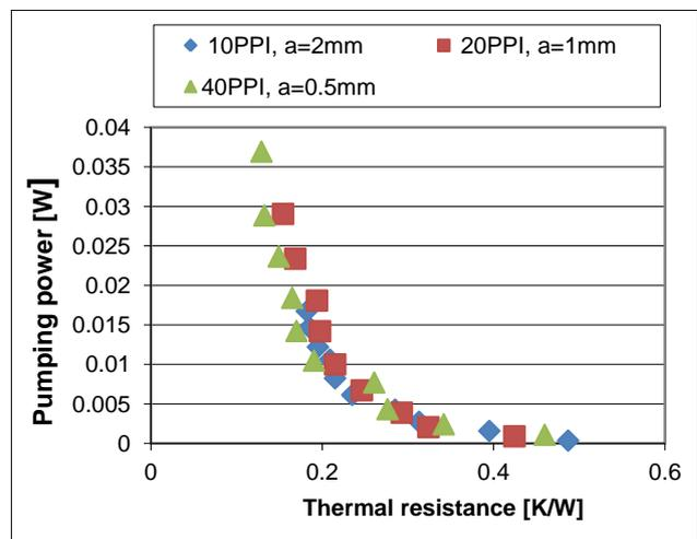
Fig. 14. Pumping power vs thermal resistance [13].
