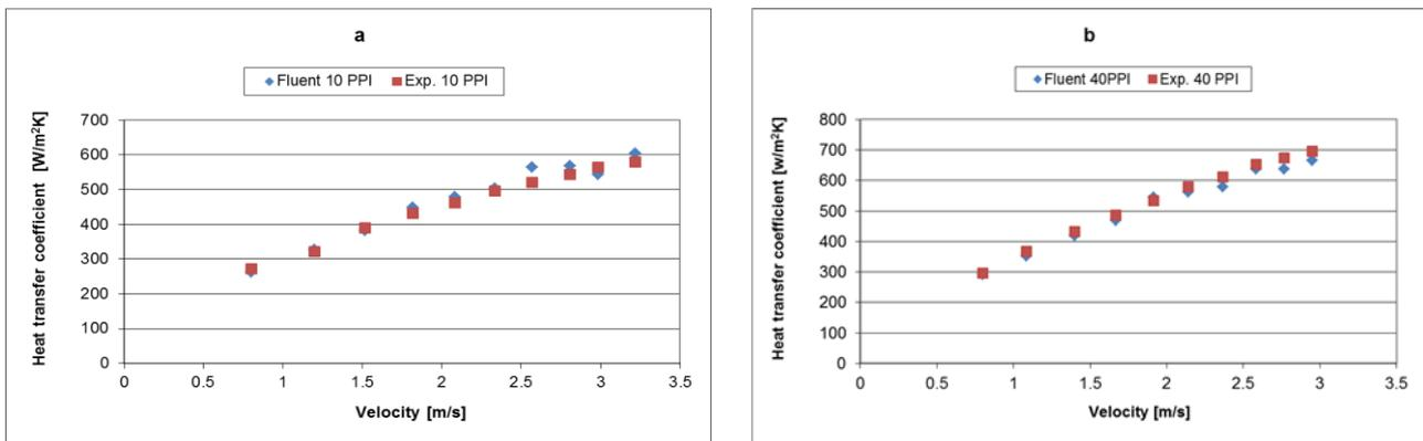
Fig. 12. Comparison between simulation and experimental heat transfer coefficient data at different velocities, for 10 and 40 porous densities and porosities  $\epsilon=0.927$ (a) and  $\epsilon=0.921$ (b) [11].
