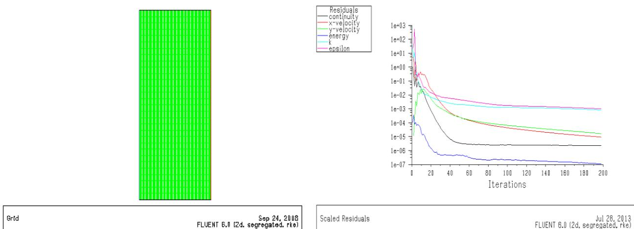
Fig. 6. Mesh (a) and plot of residuals (b) [4].
