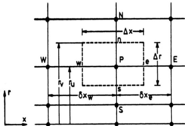
Fig. 4. Control volume for a scalar variable [6].
