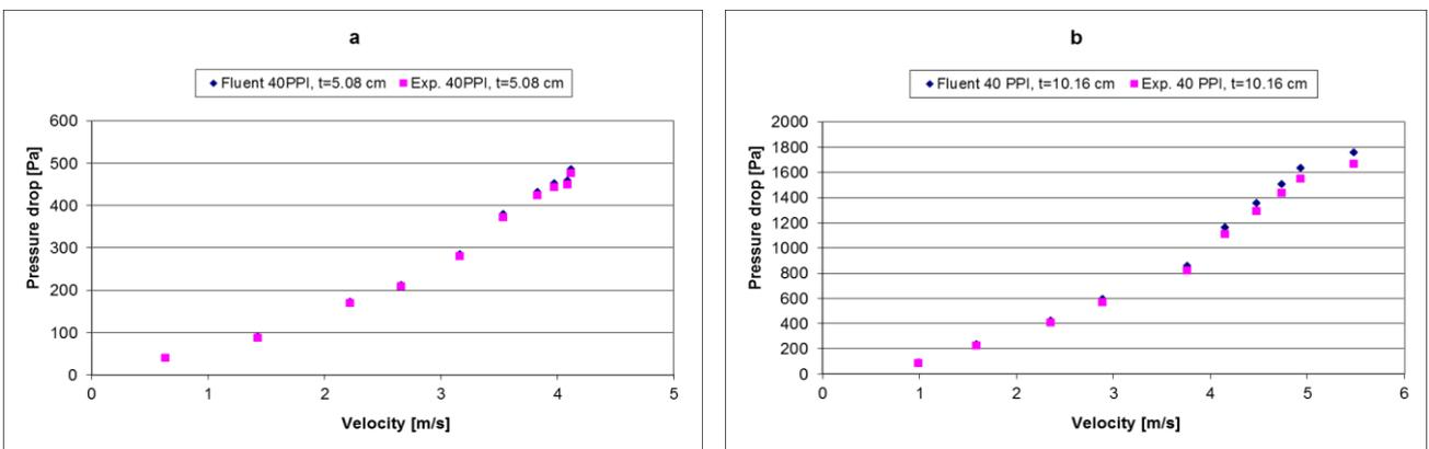
Fig. 11. Comparison between simulation and experimental pressure drop data at different velocities, for 40 PPI porous density, porosity  $\epsilon=0.927$  and heat exchanger thickness  $t= 5.08(a)$  and  $10.16(b)$  [11].
