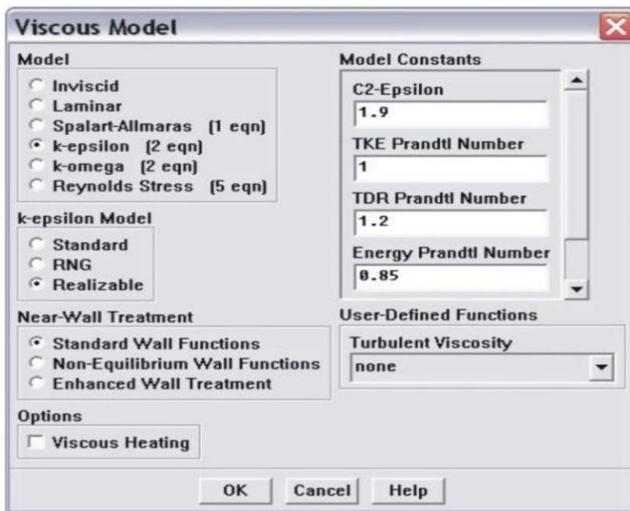
Fig. 9. Constants used in the k-ε turbulence model [5].
