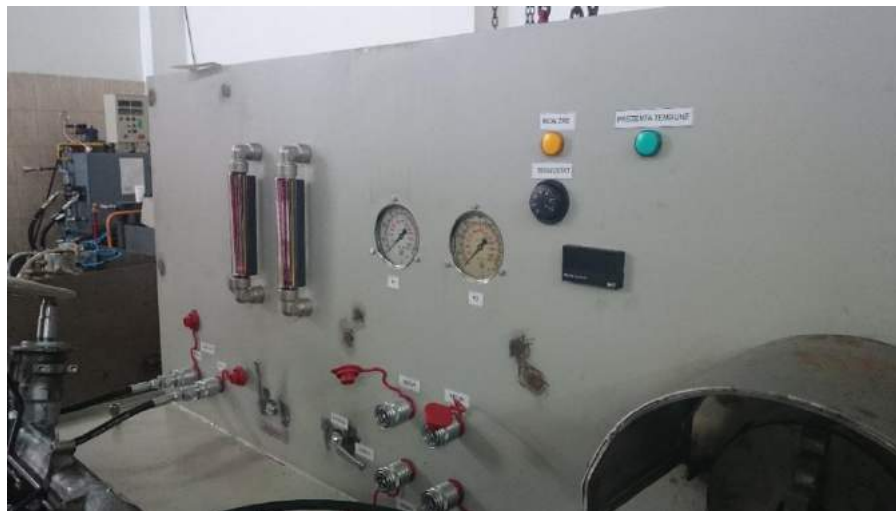
Fig. 2. Front panel of steering box testing stand
