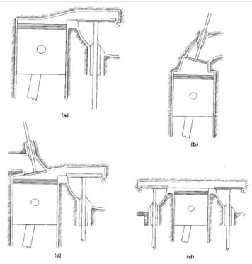
Fig. 4. Engine classification by valve location
