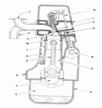
Fig. 6. Parts of Engine – Cross section of four-stroke cycle S1 engine showing engine components; (A) block, (B) camshaft, (C) combustion chamber, (D) connecting rod, (E) crankcase, (F) crankshaft, (G) cylinder, (H) exhaust manifold, (I) head, (J) intake manifold, (K) oil pan, (L) piston, (M) piston rings, (N) push rod, (0) spark plug, (P) valve, (Q) water jacket.
