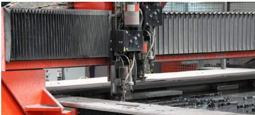
Fig. 1. Abrasive water jet cutting machine used: Bystronic ByJet Pro L
