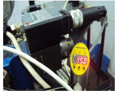
Fig. 11. Pressure transducers and pressure control valve
