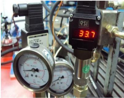
Fig. 9. Pressure transducers with display
