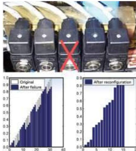
Fig. 5. Digital control reconfiguration in case of failure of a digital electrovalve [3]
