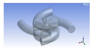
Fig. 4. Adduction channel and turbine model
