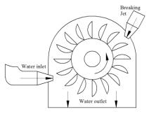
Fig. 1. Schematically representation of PELTON turbine
