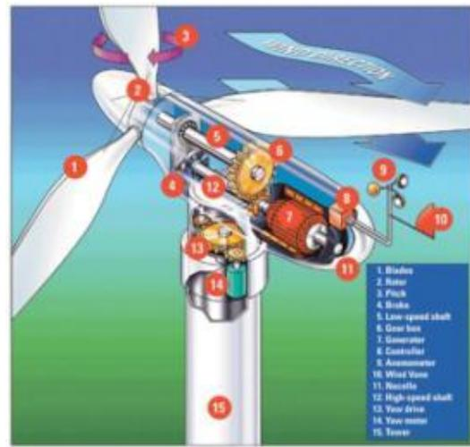
Fig. 3. The structure of a wind power station [5]
