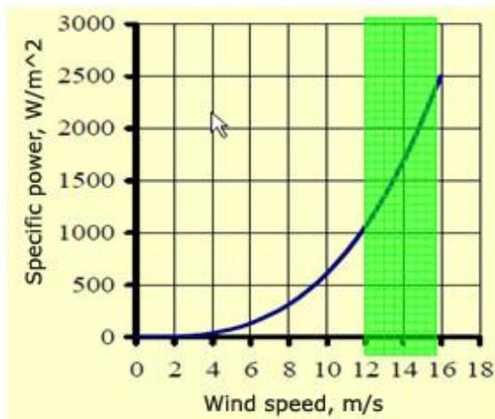
Fig. 4. Variation of specific airflow power [1]
