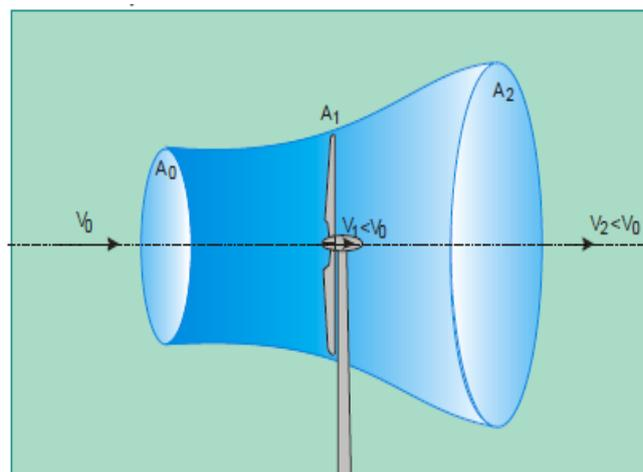
Fig. 5. Turbine effect on the airflow [1]
