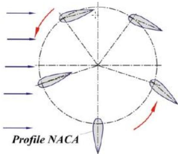
Fig. 12. Diagram of hydrodynamic profile adjustable blade rotor [1]
