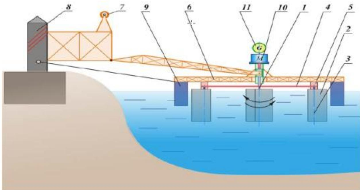
Fig. 11. Floating micro-hydropower plant with blade orientation mechanism [1]
