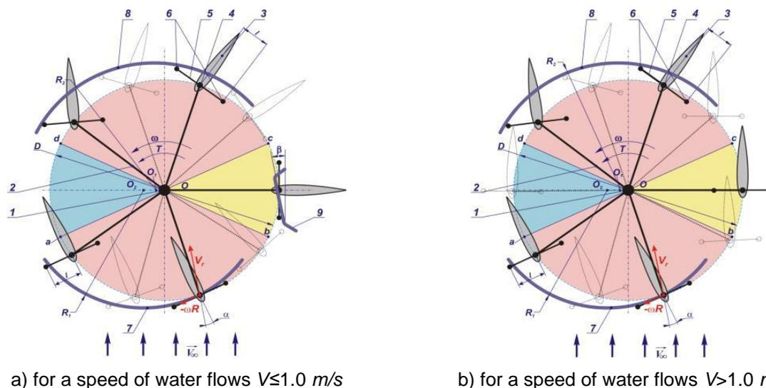
Fig. 14. Diagram of the mechanism for continuous blade orientation relative to the direction of flow [8]
