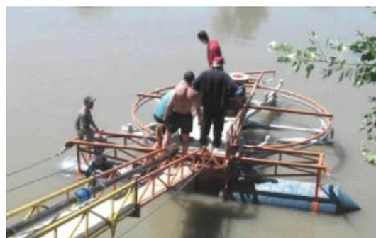
Fig. 16. The industrial prototype of the micro-hydro power plant installed on the Prut River [9]
