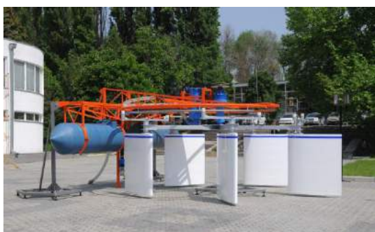
Fig. 15. Micro-hydropower plant with vertical rotor and blade with hydrodynamic profile [9]
