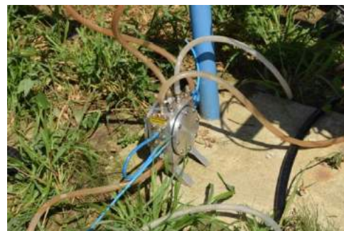
Fig. 8. Branching of the injection device to the local watering system
