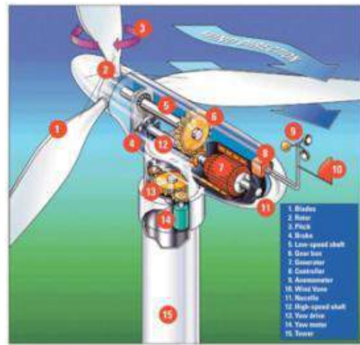
Fig. 3. The structure of a wind power station [5]
