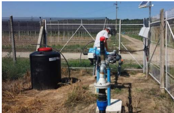
Fig.1 Fertigation system for intensive fruit plantations
