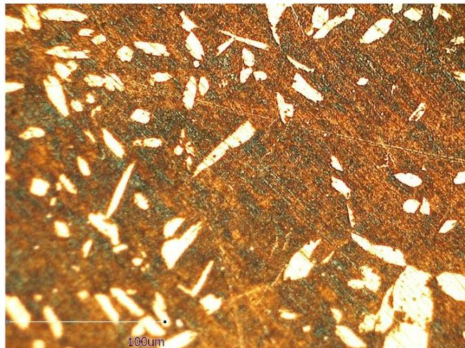
**Fig. 5.** Microstructure of the bronze CuAl10.5Ni5Fe4.8Mn1.5 (1750 x)
