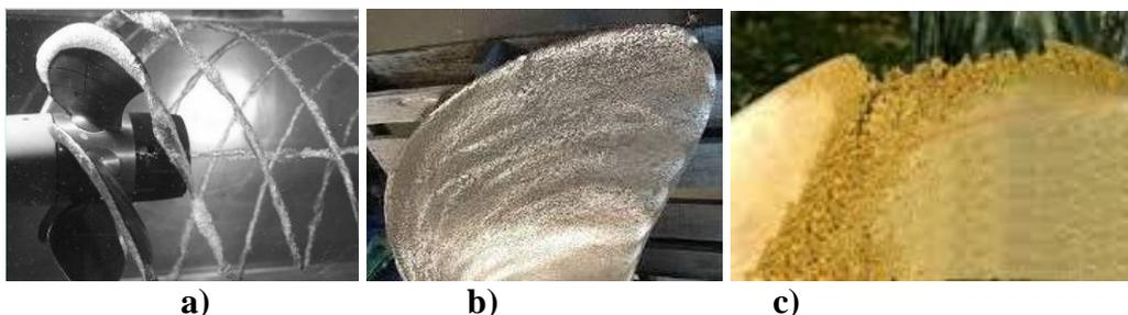
**Fig. 1.** Ship propellers running in cavitation and a blade eroded by cavitation [11]
