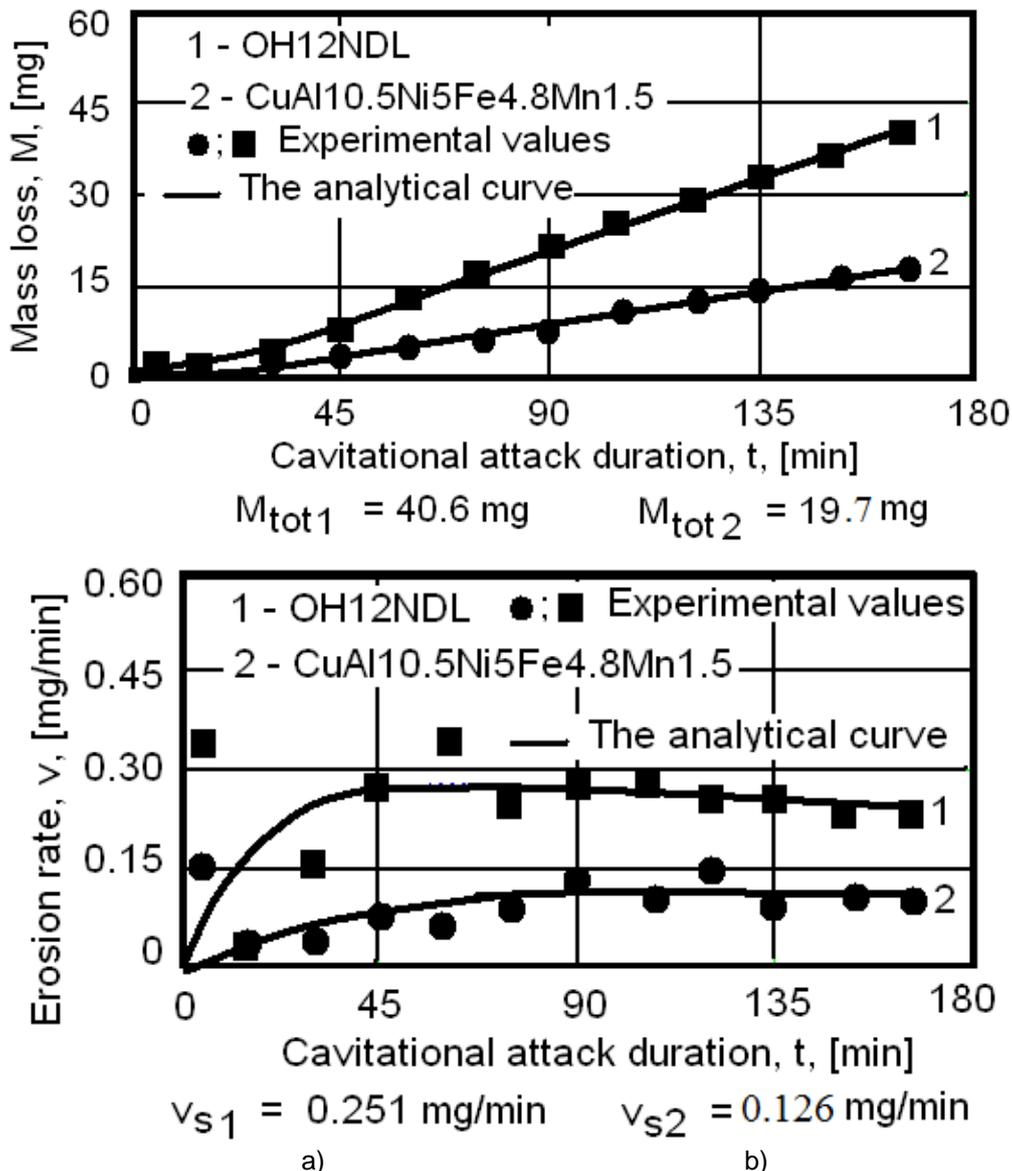
Fig. 4. Comparison with OH12NDL etalon steel:
