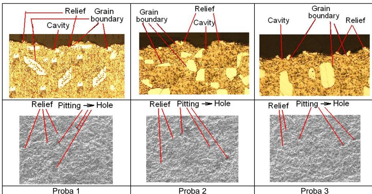
**Fig. 6.** Images of structure degradation (pitting, hole, deformations) Final exposure time, 165 minutes (1750x)
