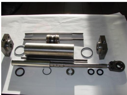
Fig. 4. Component of the cylinder for testing piston-type sealing elements
