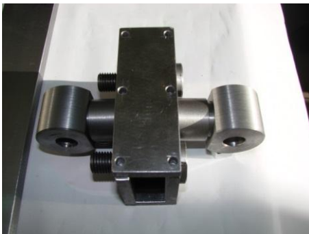
Fig. 8. Coupling for connecting the rods of the cylinders in the structure of the device
