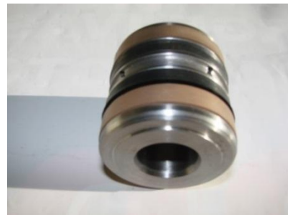
Fig. 5. Special construction piston on which the piston- type seals are mounted
