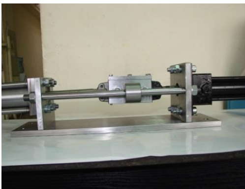
Fig. 10. Device for testing piston-type seals, assembled
