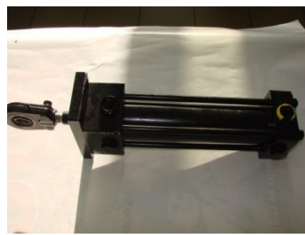
Fig. 7. Standard hydraulic cylinder D_p 50-code CH 16U050/22-145.4.HM3.0
