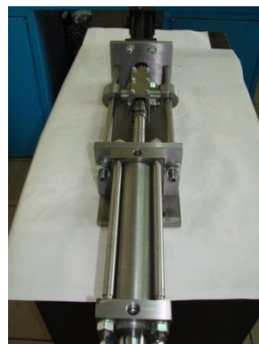
Fig. 10. Device for testing piston-type seals, assembled
