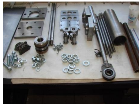
Fig. 9. Components of the device for testing of piston-type sealing elements, before assembly
