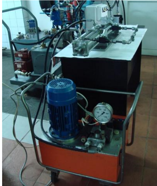
Fig. 11. Stand for testing piston seals of hydraulic cylinders
