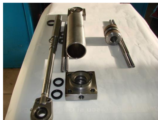
Fig. 4. Component of the cylinder for testing piston-type sealing elements
