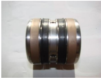
Fig. 5. Special construction piston on which the piston- type seals are mounted
